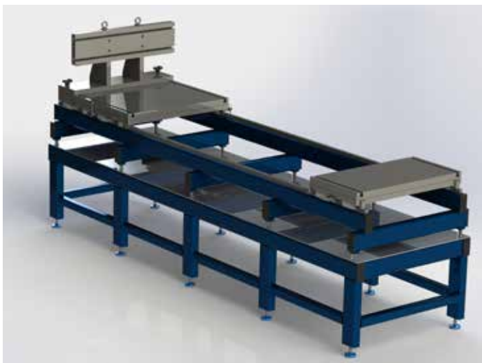
TANDEM SLIDE MOVING TABLE WITH MECHANICAL BRACKETS
